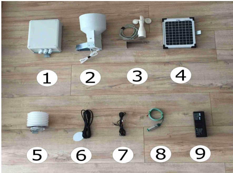
Fig. 2. Precision apiculture system sensors
